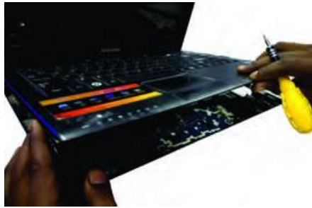
Fig. 60: Separate palm rest from bottom case
