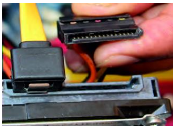
Fig. 40: Unplug 15-pin connector from HDD
