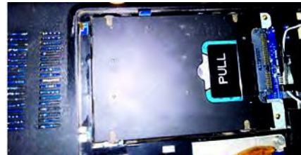
Fig. 62: Open the connector and release hard drive cable
