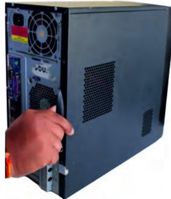
Fig. 2: Pull cabinet side cover
