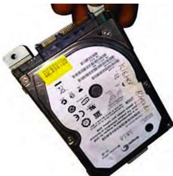
Fig. 63: Remove hard drive assembly
