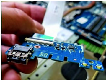
Fig. 66: Remove USB LED status board
