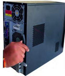
Fig. 39: Pull cabinet side cover
