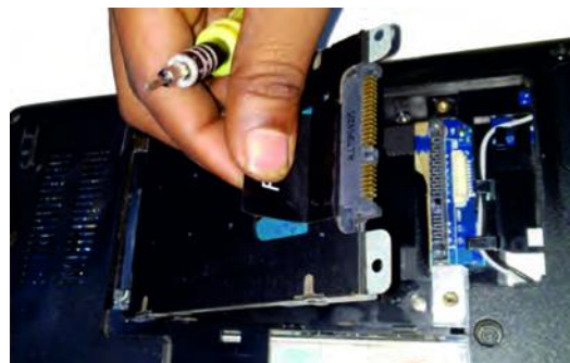
Fig. 64: Disconnect SATA cable
