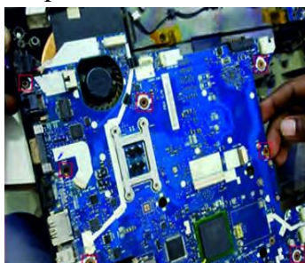
Fig. 73: Disconnect cables from motherboard and remove screws
