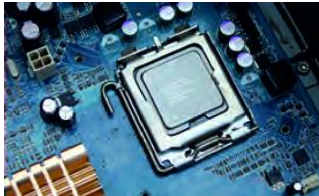
Fig. 5: Installing CPU on the motherboard
