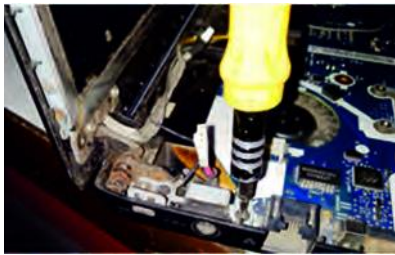
Fig. 71: DC power jack mounted under display hinge
