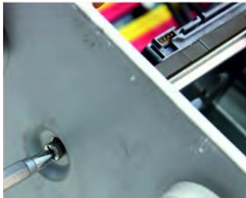
Fig. 13: Tighten screws of HDD
