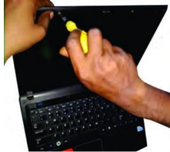
Fig. 77: Remove the four screws securing LCD screen
