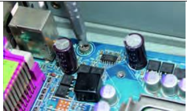
Fig. 11: Tighten all the motherboard screws
