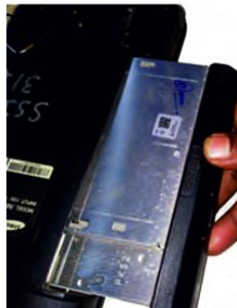
Fig. 67: Remove optical CD DVD drive connector board
