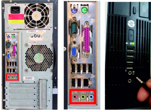
Fig. 26: Connecting speakers or headphones, and microphone
