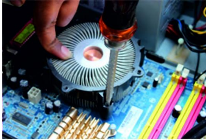
Fig. 44: Unscrew heat sink
