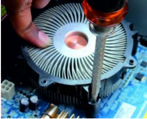
Fig. 7: Screw the heat sink
