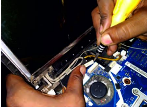
Fig. 80: Disconnect video cable from screen
