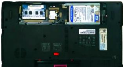
Fig. 61: Remove screws from the hard drive and disconnect it
