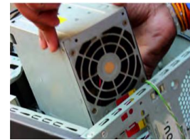
Fig. 50: Unscrew the SMPS and remove it from cabinet
