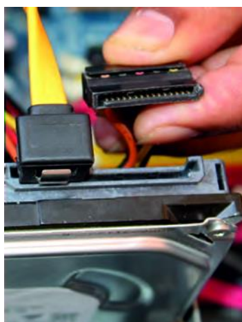
Fig. 20: Plug-in 15-pin connector to HDD
