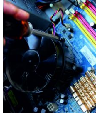
Fig. 8: Screw the heat sink fan assembly
