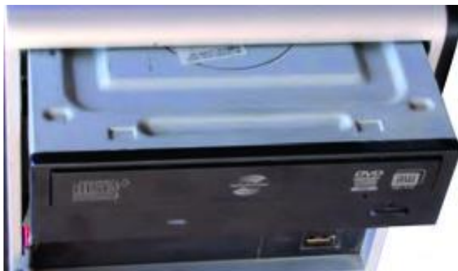
Fig. 14: Insert optical drive
