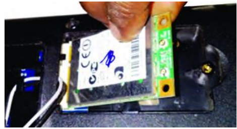
Fig. 72: Disconnect Wi-Fi Module
