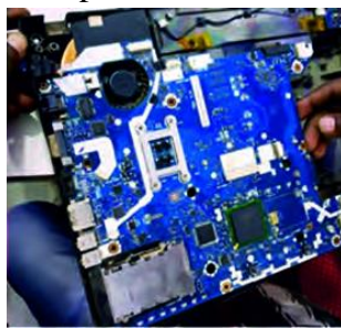
Fig. 74: Remove the motherboard from notebook case
