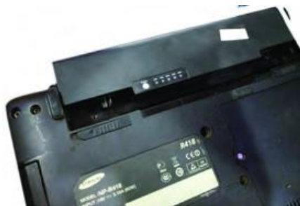
Fig. 59: Remove battery and optical drive
