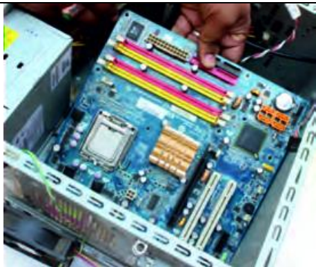
Fig. 10: Lay the motherboard over the standoffs
