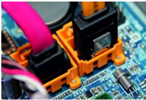
Fig. 48: Unplug power cable
