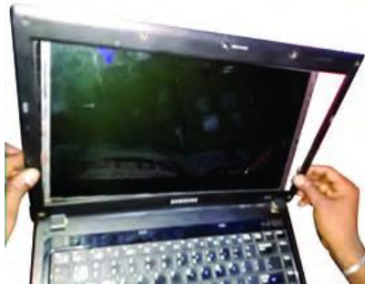
Fig. 76: Notebook PC LCD screen removal
